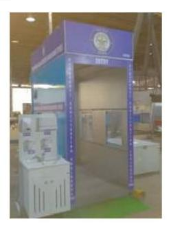
The system consists of roof mounted and bottom tanks with a total of 700 liters capacity. Approximately 650 personnel can pass through the chamber for disinfection until the refill is required.
