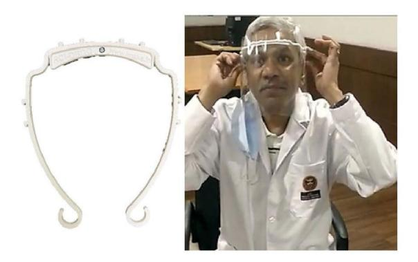
The holding frame is manufactured using Fused Deposition Modeling (3D printing). Polylactic Acid filament is used for 3D printing of the frame. This thermoplastic is derived from renewable resources such as corn starch or sugarcane and is biodegradable. The face mask will be mass produced using injection moulding technique for volume production.
